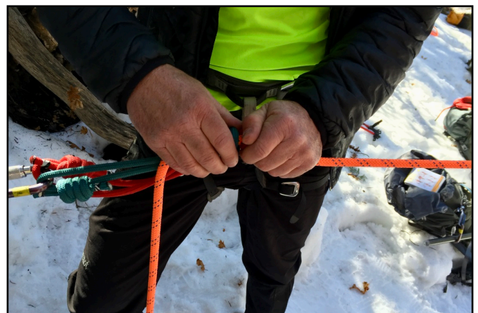
Two prusiks tied onto the belay line, and clipped into their own anchor, which a team member will keep a bit loose during a lower but which should seize on their own and hold the belay line if the main line fails. Gloves might be a good idea here.
