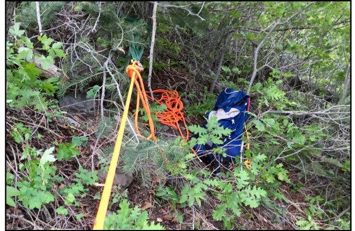
A “wrap three, pull two” webbing anchor on a tree, with a Scarab lowering device clipped into a 27kn+ biner on the anchor, theoretically providing a 10 to 1 safety margin on the main line’s expected rescue load (UCSSAR uses a static safety factor).
